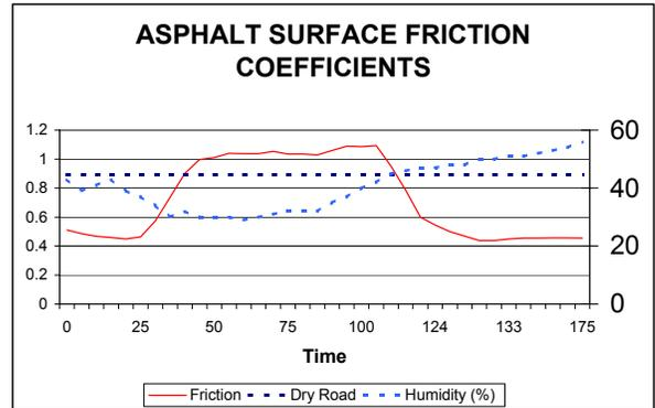
As the graph illustrates, an asphalt surface treated with Caliber M1000 provides a friction coefficient only slightly less than that of a water-wet road. In addition, once allowed to dry, the Caliber M1000 provided a friction coefficient greater than that of the dry asphalt! Further more, the Caliber M1000 treated surface did not experience the "slickness window" that other liquid products may.
